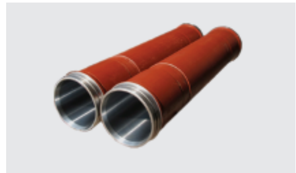
Concrete delivery cylinder is 200mm diameter, and stroke is 1000mm, bigger and higher capacity; inwall is covered with high chrome, more wearable and longer service life;
